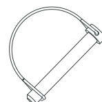
SP-1 SECURING PIN (4x)
